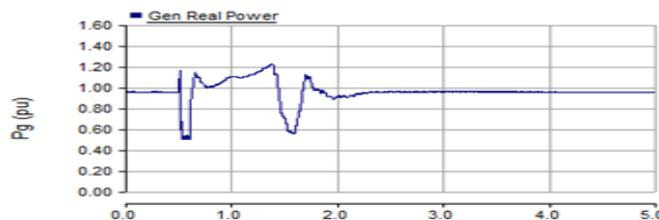
Fig. 10a. Generator's active (Pg) output.
